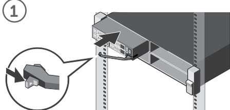
Beginning from the top, install the sled(s) into the enclosure, from left to right.
